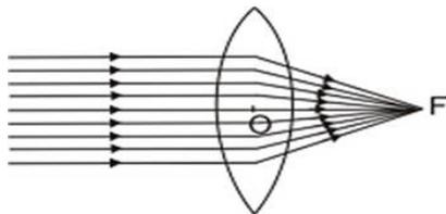
Object at infinity. Image at F on the other side of lens.
