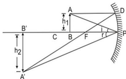
Magnification is positive when image is erect and virtual. Magnification, m is negative when image is inverted and real.
