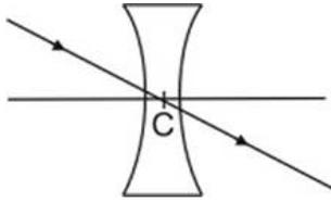
Rule 2. An incident ray passing through optical centre of a concave lens goes straight after passing through the concave lens.
