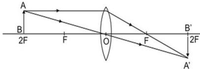
Object at  $2F$ , image at  $2F$  on the other side of the lens. Image is of size same as that of the object. When the object is between  $F$  and  $2F$ , its real, inverted, magnified image is formed on the other side of the convex lens as shown in fig.
