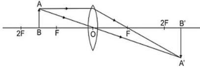
Object between  $F$  and  $2F$  real, inverted, magnified image is formed beyond  $2F$  on the other side of lens.
